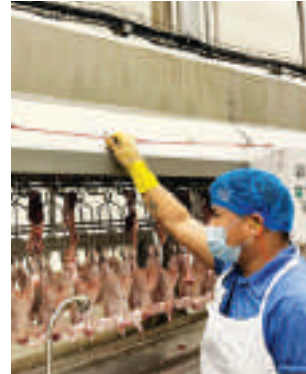
Safety Pull Cords at High-risk areas
